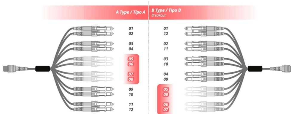
These fibers are not used on MPO8 configuration /
